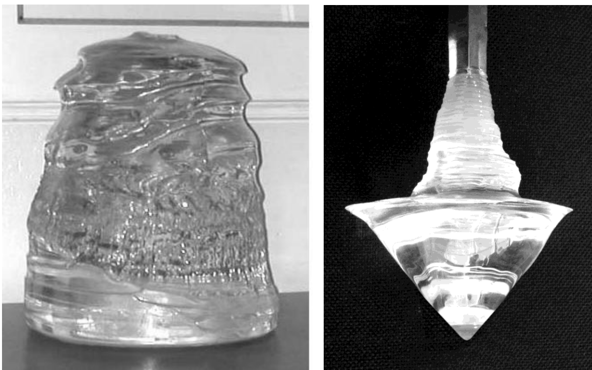
Fig. 1. Sapphire boule with a diameter up to 300 mm and 65 kg weight, grown by Monocrystal Inc. in Stavropol (Russia) using the Kyropoulos technique (left) and the sapphire crystal photo at an intermediate growth stage (right).
